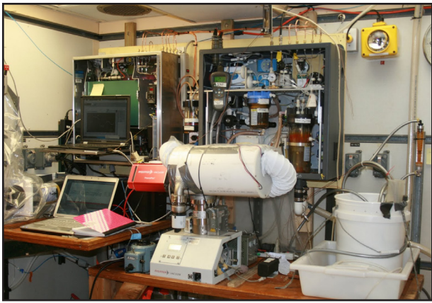
An experimental set up for measuring seawater carbon dioxide (CO 2 ) aboard the R/V Thomas G. Thompson. Credit: Jessica Cross/NOAA
