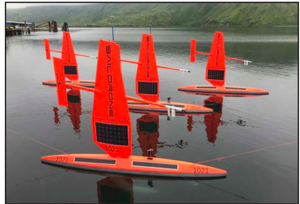
Saildrones, capable of making autonomous ocean measurements, waiting at the dock in Dutch Harbor, Alaska before their multi-month NOAA research mission. Credit: Saildrone, Inc.
