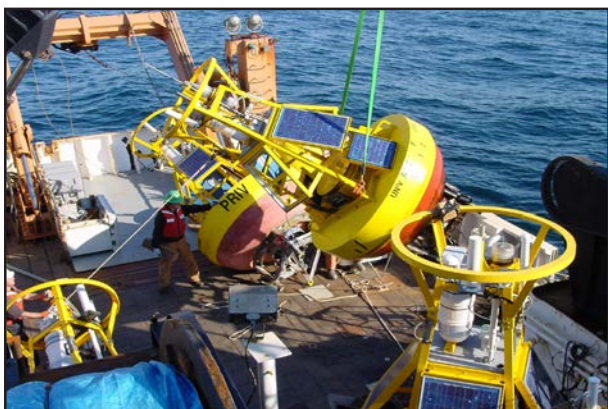
An ocean mooring in the Gulf of Maine used to monitor ocean conditions. Credit: Personnel of NOAA Ship DELAWARE II
