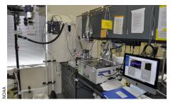
**Burke-o-Lators:** Often co-located at hatcheries, these high-accuracy systems analyze multiple OA parameters and provide a clear picture of real-time conditions. Burke-o-Lators are located in Seward, Kodiak, and Sitka.
