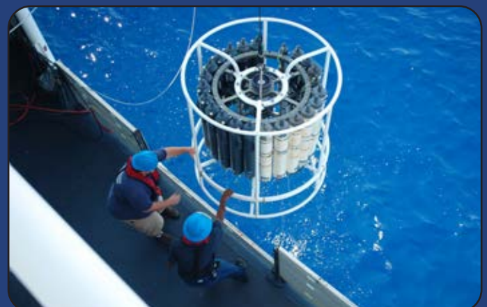
Scientists collect water samples to measure ocean acidification from a NOAA vessel.
